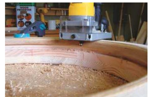
▲ Pic.14 Check the fit of the beading in the frame, then add a profile with a rounding over bit
